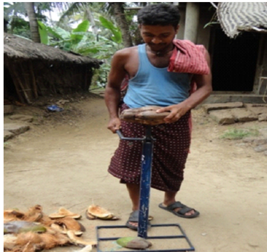
Dehusking with coconut dehusker (standing type)
