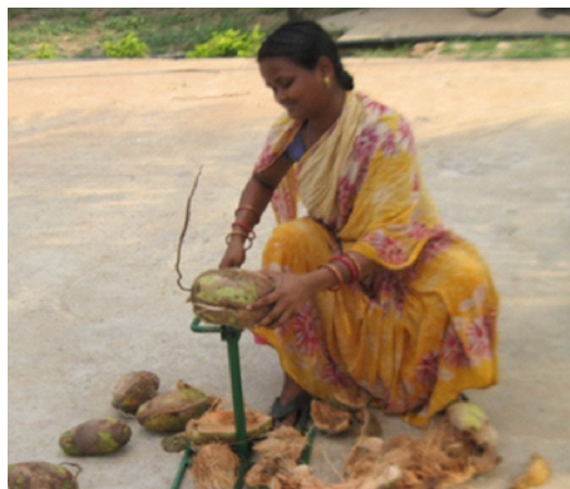
Dehusking with coconut dehusker (standing type)
